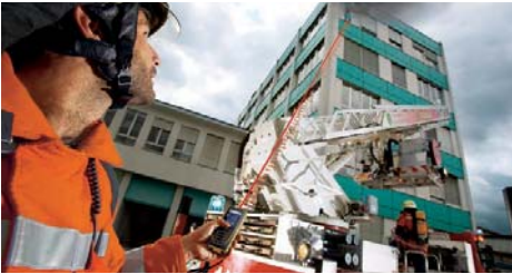
Fire brigade – indirect height measurement with the Pythagoras function
