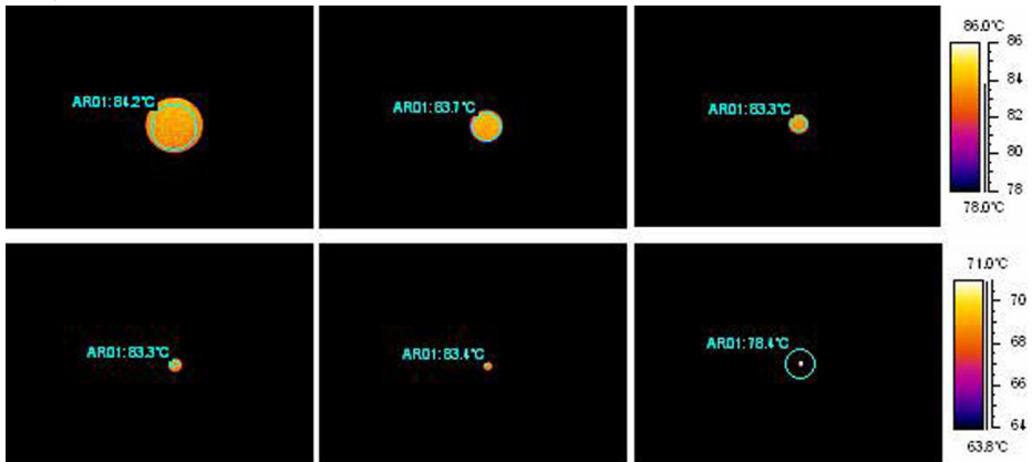
Figure 28.20 Temperature readings from a blackbody at +85°C (+185°F) at increasing distances (24° lens)
