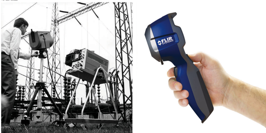
Figure 26.1 LEFT: Thermovision® Model 661 from 1969. The camera weighed approximately 25 kg (55 lb.), the oscilloscope 20 kg (44 lb.), and the tripod 15 kg (33 lb.). The operator also needed a 220 VAC generator set, and a 10 L (2.6 US gallon) jar with liquid nitrogen. To the left of the oscilloscope the Polaroid attachment (6 kg/13 lb.) can be seen. RIGHT: FLIR i7 from 2009. Weight: 0.34 kg (0.75 lb.), including the battery.
