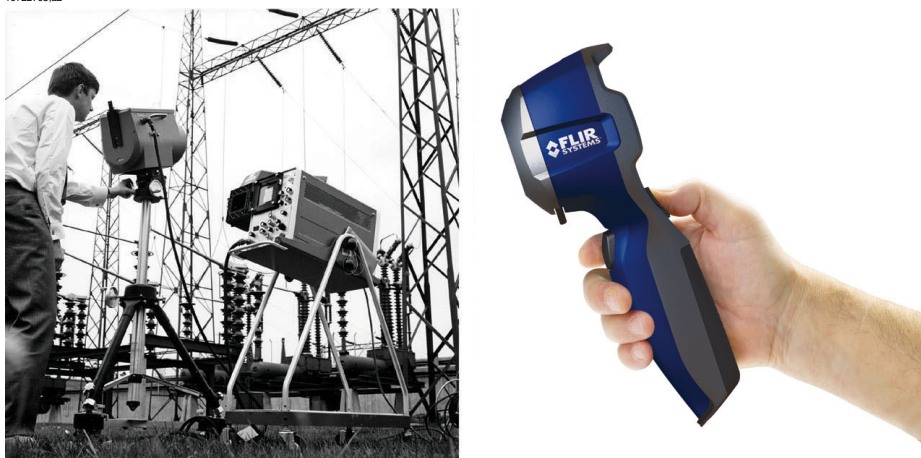
Figure 32.2 LEFT: Thermovision® Model 661 from 1969. The camera weighed approximately 25 kg (55 lb.), the oscilloscope 20 kg (44 lb.), and the tripod 15 kg (33 lb.). The operator also needed a 220 VAC generator set, and a 10 L (2.6 US gallon) jar with liquid nitrogen. To the left of the oscilloscope the Polaroid attachment (6 kg/13 lb.) can be seen. RIGHT: FLIR i7 from 2009. Weight: 0.34 kg (0.75 lb.), including the battery.
