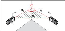
Press the key **two times** - the triangle symbol appears in the display.
