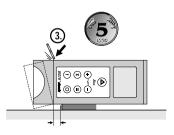
By pressing downwards at an angle and to the front simultaneously, the battery compartment can be easily opened.
