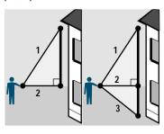
For estimating the height of buildings. Very useful for making measurements from standing position (no bending) if the height is determined with three distances.
