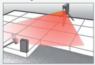
A sensor detects the laser line at distances of up to 30 m. This makes it easy to monitor the laying of terrace tiles, for example. The self-levelling function can be switched off at any time (locking function), and the laser line can be projected into any location.
